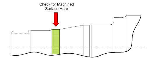
If the surface is machined, no further action is necessary. Install hub according to step 10.
